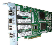
AD393A HP PCIe 2p 4Gb/s FC and 2p 1000SX HBA
