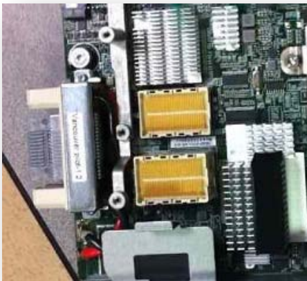
Figure A-1 – Showing the mezzanine card slots (gold-colored) in a BL460c G7 server blade
