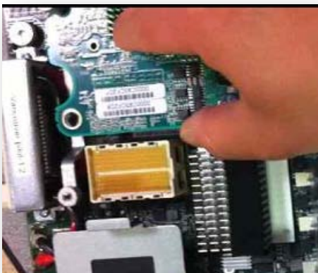
Figure A-2 – Installing an HBA
